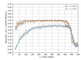
Figure 3: Efficiency of the energy transfer from the charge-pump output capacitor  $C_S$  to the output capacitor  $C_0$ , versus initial voltage across  $C_S$  and for two values of the initial voltage across  $C_0$ .
