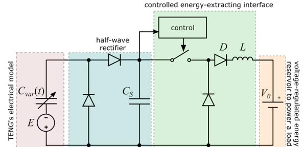
Figure 1: Sketch of the complete TENG-based kinetic energy harvesting system considered in this paper. The different parts are highlighted: the electrical lumped-model of the TENG, the half-wave conditioning circuit, and the energy-extracting interface.
