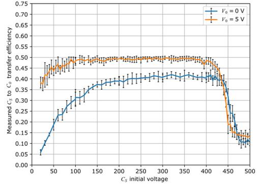
Figure 3: Efficiency of the energy transfer from the charge-pump output capacitor  $C_S$  to the output capacitor  $C_0$ , versus initial voltage across  $C_S$  and for two values of the initial voltage across  $C_0$ .
