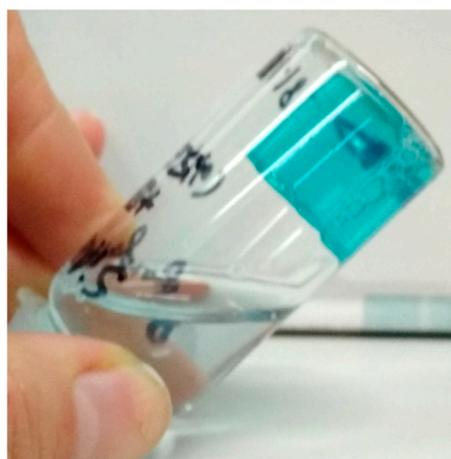
**Figure 7.** Brilliant Blue adsorption by SF hydrogel at pH 3. In contrast to MB, BB can be completely adsorbed at pH 3.
