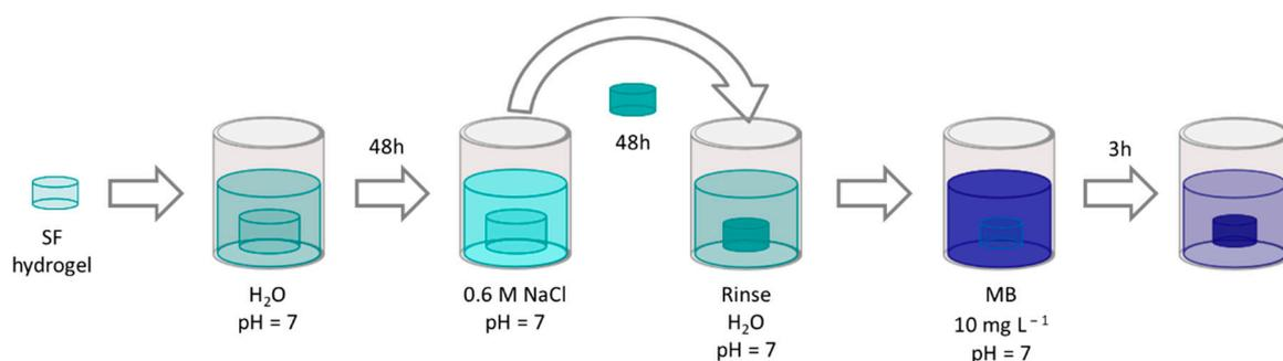
**Figure 1.** Schema of the procedure followed to evaluate the effect of salt pretreatment on the SF hydrogel MB adsorption capacity. After formation, the hydrogel is immersed in water for swelling, then in a 0.6 M NaCl solution until hydrogel saturation (6 days). The hydrogel is then rinsed and immersed in  $10 \text{ mg L}^{-1}$  MB solution for MB absorption.
