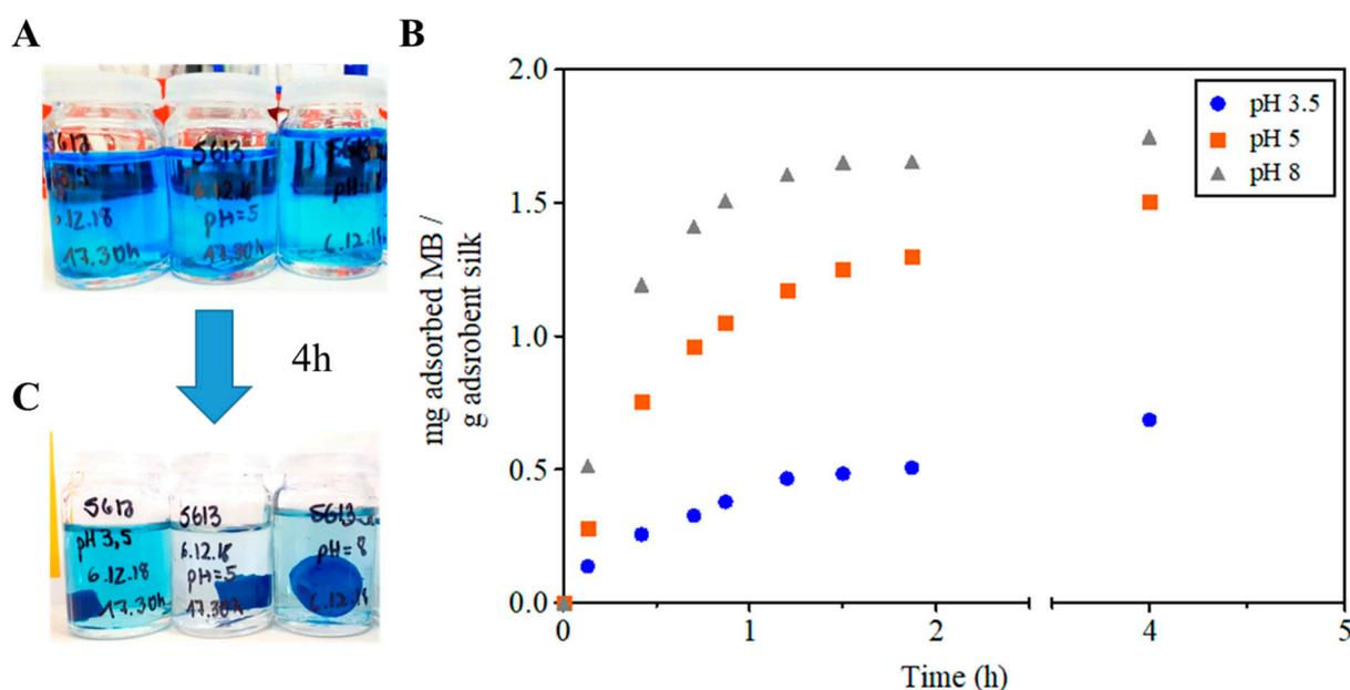
**Figure 5.** MB adsorption by SF hydrogels after three different pH treatments. Initial (A) and final (C) images of pH-treated silk hydrogels submerged in methylene blue solutions. From left to right, the pH treatments were 3.5, 5 and 8, respectively, in both images. Quantitative analysis of the mass of methylene blue adsorbed over time by UV-Vis spectrometry at 664 nm (B).
