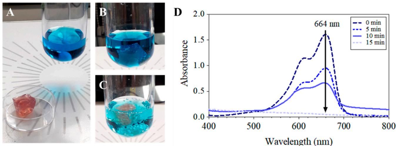
**Figure 9.** Silk-Au NPs hydrogel bionanocomposite and MB solution (A), image taken at the start (B) and during (C) MB reduction reaction. The formation of  $H_2$  results in gas bubbles entrapped within the silk-Au NPs hydrogel. MB reduction kinetics monitored by UV-vis spectrophotometry (D).
