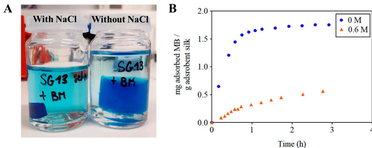
**Figure 6.** Images of sodium chloride treated (**left**) or not (**right**) SF hydrogels after MB adsorption (A). After salt pretreatment, the SF hydrogel was considerable shrunk. MB adsorption kinetics after sodium chloride pretreatment (B).
