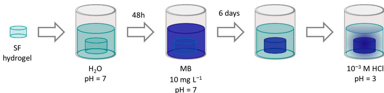
**Figure 2.** Schema of the procedure followed to evaluate SF hydrogel MB release. After formation, the hydrogel is immersed in water for swelling, then in a MB solution until hydrogel saturation (6 days). The MB-saturated hydrogel is then immersed in 10<sup>-3</sup> M HCl solution for MB release.
