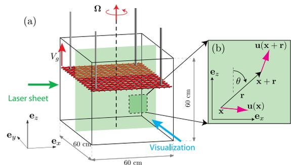
FIG. 1 (color online). (a) Experimental setup. The water-filled tank is rotating at  $0 \leq \Omega \leq 1.68 \text{ rad s}^{-1}$ . The grid is towed from the bottom to the top, and PIV measurements are performed in the vertical plane  $(x, z)$  in the rotating frame during the turbulence decay. (b) Definition of the vector velocity increment  $\delta \mathbf{u} = \mathbf{u}(\mathbf{x} + \mathbf{r}) - \mathbf{u}(\mathbf{x})$ .
