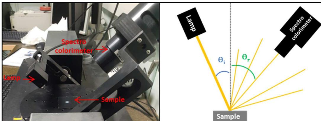
Figure 2 : Photograph and scheme of the goniospectrophotometer.
