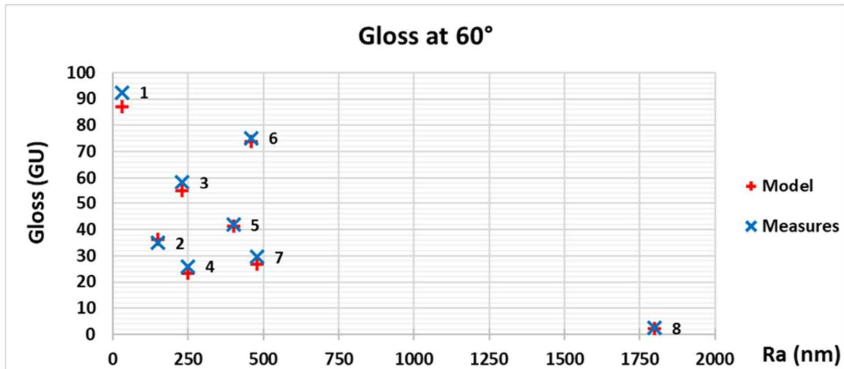
Figure 10 : Gloss at 60° as a function of the arithmetical mean roughness Ra.
