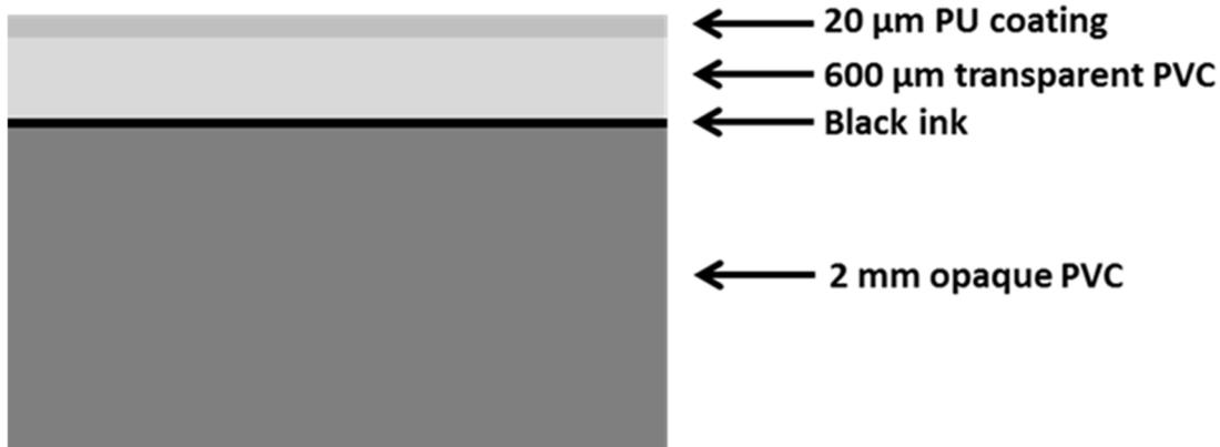
Figure 1 : Structure of the material.
