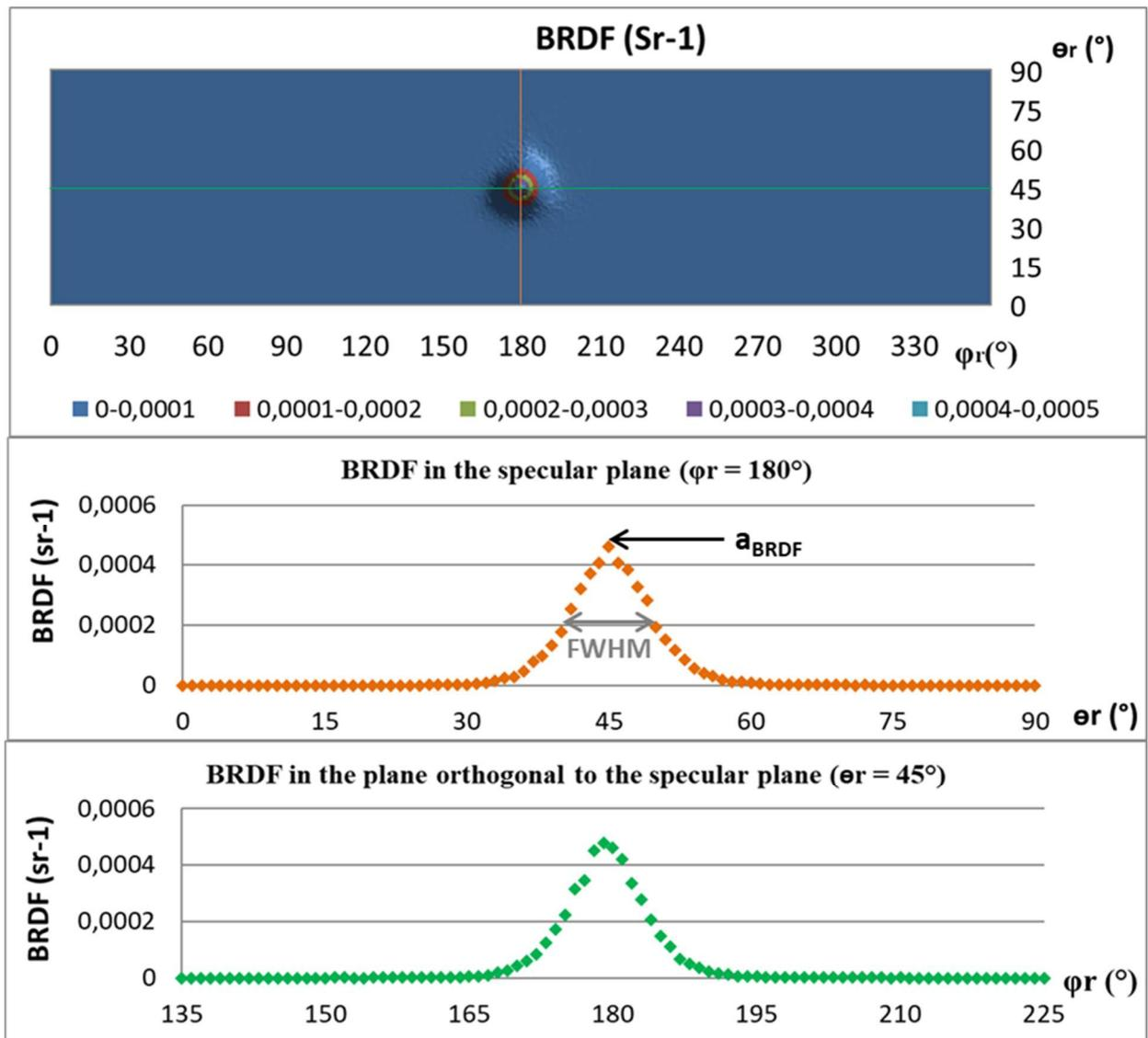
Figure 5 : BRDF computed for sample 5 with an increment of  $1^\circ$ . 3D BRDF (a), cross-section in the specular plane (b), cross-section in the plane orthogonal to the specular plane which contains the specular direction (c). The colours of symbols in b) and c) correspond to the colours of the cutting planes in a).
