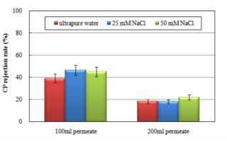
Figure 3. Influence of ionic strength on CP retention by NF.
