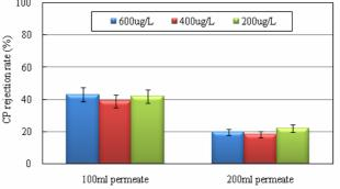
Figure 2. Influence of CP feed concentration on CP retention by NF.
