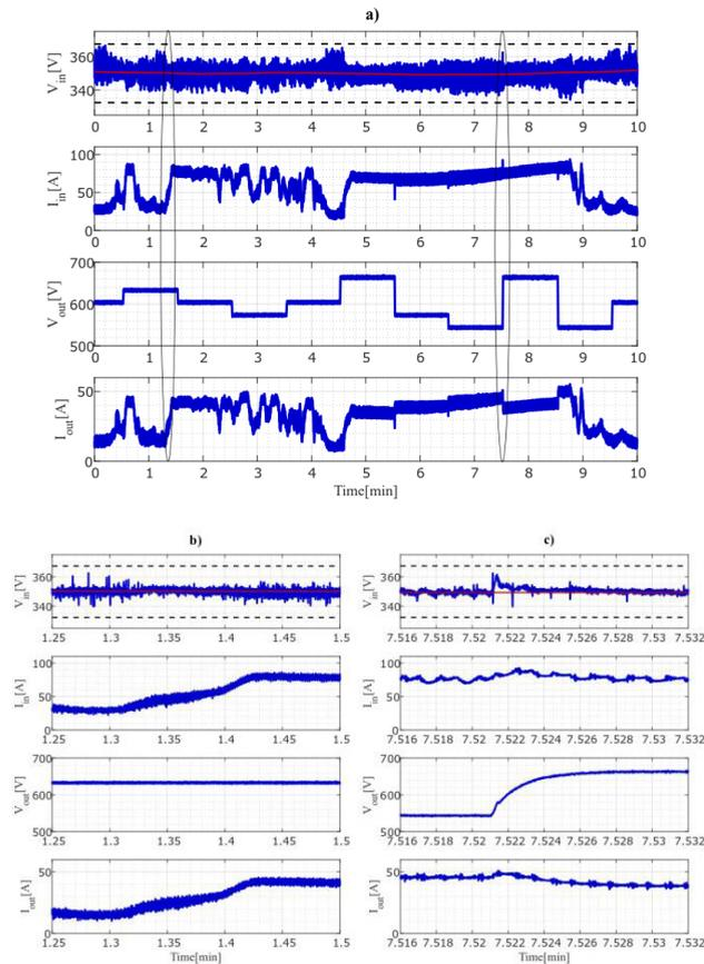
**FIGURE 18.** Experimental waveforms: a) Input voltage  $V_{in}$  regulated to 350 V, input current  $I_{in}$  following the PV profile for maximum power of 30 kW, output voltage  $V_{out} = 600$  V with step variations in the range  $\pm 10\%$  of output voltage, output current  $I_{out}$ . b) Zoom on input current change from 30 A to 80 A. c) Zoom on output voltage change from 540 V to 660 V.
