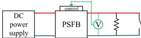
FIGURE 16. Test bench set-up for short-circuit tests.
