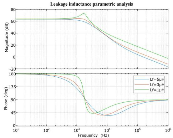
FIGURE 7. Bode diagram of PSFB transfer function  $H_2$ , with parameters from Table 2 and different values of leakage inductance  $L_f = 5 \mu\text{H}$  (blue),  $L_f = 3 \mu\text{H}$  (red),  $L_f = 1 \mu\text{H}$  (green).
