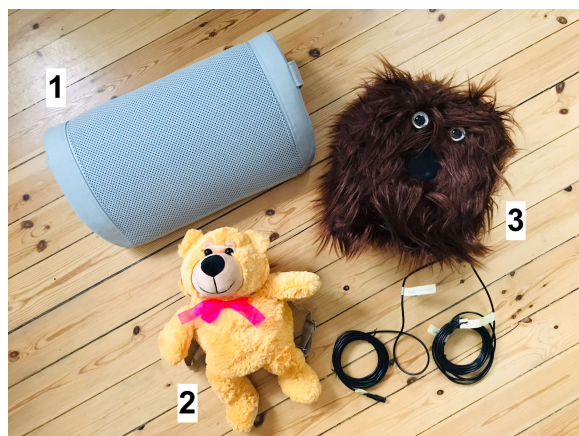
Figure 3. The Haptic Music Players (HMPs) used in the study: HMP (1) a haptic pillow, HMP (2) a plush toy backpack with an embedded haptic strap, and HMP (3) a custom-built plush toy with an embedded tactile transducer and full-range speaker.
