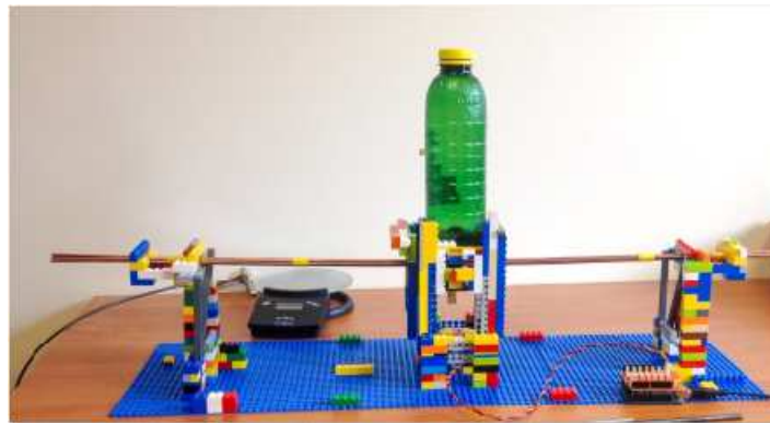
Figure 2: experimental setup of the project studying the deformation of a metallic rod with fixed extremities. The water bottle stands on a platform that is free in the vertical direction. By adding water in the bottle, the weight applied on the rod increases. A magnet is attached at the middle of the rod, and a Hall sensor is fixed on the table below to measure the vertical deformation when the force is increased.
