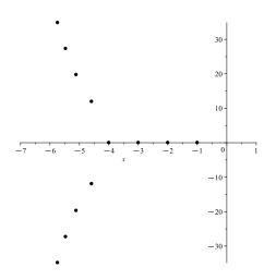
Fig. 1. Spectrum distribution of the closed loop system (1) using a delayed PD controller (2).
