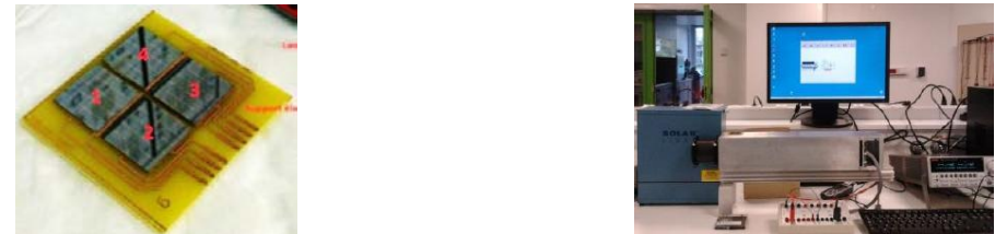
Figure 2. Left: 4 silicon photovoltaic (PV) cells of 3.24 \text{cm}^2 , glued with a conducting paste on a test PCB. Right: Automated test bench for I(V) measurements of the PV cells, in obscurity or under lighting.
