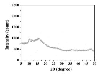
Fig. 5 Representative XRD profile of the Gloecapsa gelatinosa EPS sensor membrane
