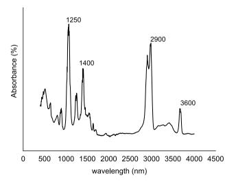
$\begin{tabular}{ll} Fig. 4 & Infrared spectra of the Gloecapsa gelatinosa EPS sensor membrane \\ \end{tabular}$
