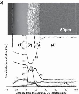
**Fig. 1.** Microstructure and chemical composition of the as-processed systems without (a) and with a DB (b).
