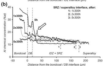
Fig. 4. Evolution of the Al chemical concentration profiles in systems without (a) and with a DB (b) following cyclic oxidation at  $1100\,^{\circ}$ C in air.
