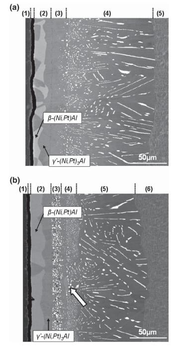
**Fig. 3.** Microstructure of the systems without (a) and with a DB (b) after 300 h isothermal oxidation at 1100  $^{\circ}$ C in air.
