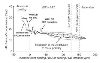
**Fig. 5.** Comparison between Al chemical concentration profiles obtained in zones containing SRZ and in zones without SRZ formation after 300 h isothermal oxidation at  $1100\,^{\circ}\text{C}$  in air.
