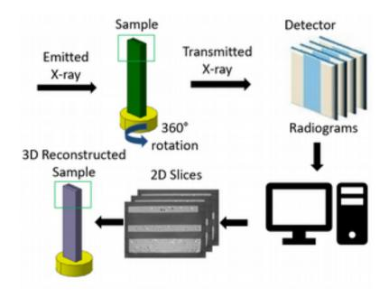
Figure 2. Principle of tomography measurements
