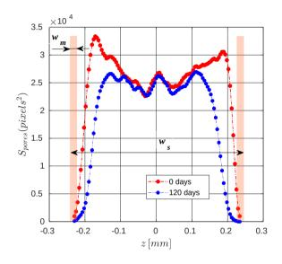
Figure 22. Evolution of the pore sections along the thickness direction in sample E2, at the initial state and after 120 days of aging
