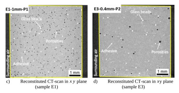
Figure 7. Reconstituted volumes of the samples obtained from the CT scan
