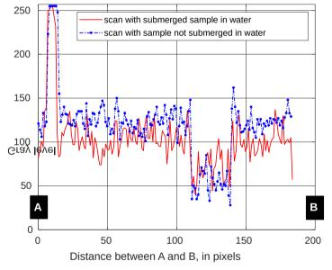
c) Gray level comparison between the two configurations on the same AB path
