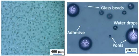
a) Sample E1 (0.4 mm thick) after curing
