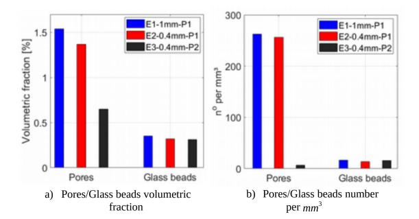
Figure 11. Volume fractions and numbers of pores and glass beads in the different samples
