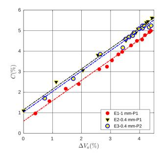
Figure 19. Mass change of the samples versus variation in the effective volume of the adhesive
