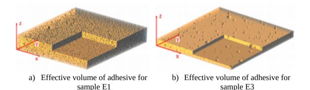
Figure 12. 3D representation of the effective volume of adhesive for samples E1 and E3
