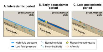
**Figure 10.** Schematic diagram of the evolution of pore fluid pressure near the trench during the postseismic period. (a) Interseismic period: fluid pressure is high as fluids are trapped at the plate interface. (b) Early postseismic period: fluid pressure is low as afterslip causes dilation and fluids escape the interface. (c) Late postseismic period: fluid pressure increases again as the afterslip slows down.
