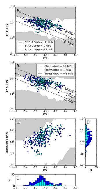
**Figure 4.** Panels (a)–(c) show source properties (corner frequencies inferred from *P*-waves and *S*-waves, stress drop) as a function of moment magnitude. Panels (d and e) show the distribution of stress drops and magnitudes respectively. Light blue represents repeaters and dark blue represents non-repeaters. The gray shaded areas show for a given magnitude the median upper and lower frequency limits between which corner frequencies can be resolved.
