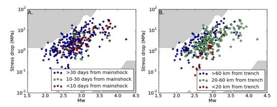
**Figure 6.** Distribution of stress drops as a function of magnitude. (a) Events colored by time. The timing of repeaters does not influence the stress drop Versus magnitude trend. (b) Events colored by distance to the trench. The gray shaded areas show for a given magnitude the median upper and lower frequency limits between which corner frequencies can be resolved.
