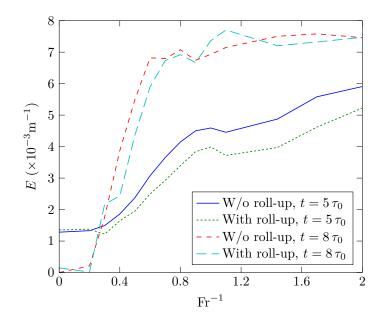
Figure 12: Comparison of vortex descent without and with a roll-up for a typical jet position of a twin-engined aircraft ( $\bar{b}_{jet} = 0.335$ )
