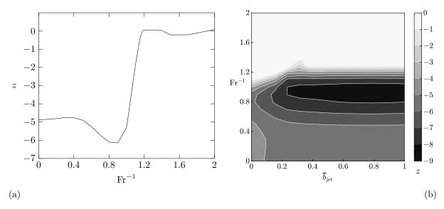
Figure 5: (a) Altitude of the vortex dipole at  $t = 5 \tau_0$  when there is no jet. (b) Altitude of the vortex dipole at  $t = 5 \tau_0$ , when there is a jet, as a function of  $Fr^{-1}$  and  $\bar{b}_{iet}$ .
