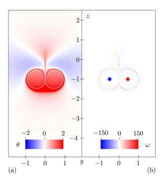
Figure 4: (a) Vorticity and (b) perturbation of potential temperature fields at  $t = 2\tau_0$  for  $Fr^{-1} = 1$ . All distances are normalized by  $b_0$ .
