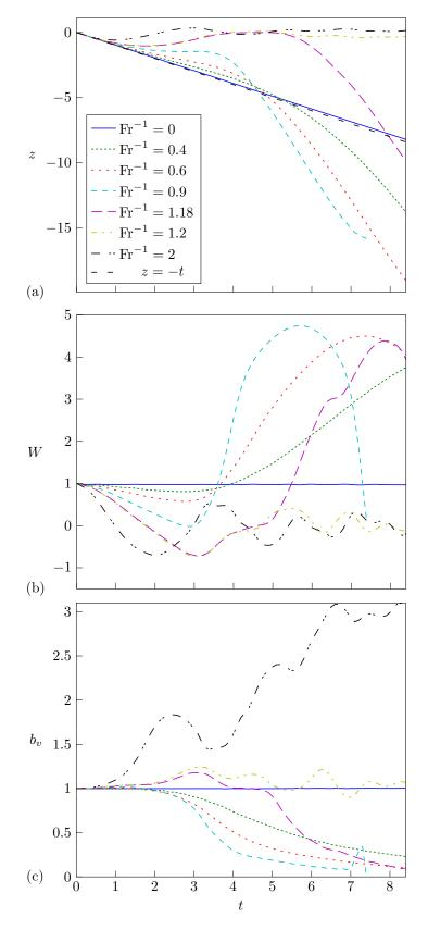
Figure 2: (a) Altitude of the vortices as a function of time for different values of  $\text{Fr}^{-1}$ . (b) Descent velocity of the pair of vortices. (c) Distance between the vortices. Distances are normalized by  $b_0$ , time by  $\tau_0$  and velocity by  $W_0 = \Gamma_0/(2\pi b_0)$ .
