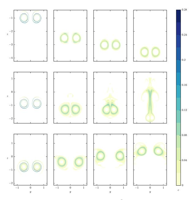
Figure 7: Evolution of the passive scalar field over time for  $\bar{b}_{jet} = 0.335$ . From top to bottom: Fr<sup>-1</sup> = 0.2, Fr<sup>-1</sup> = 1, Fr<sup>-1</sup> = 1.4. From left to right:  $t = \tau_0$ , 2.5  $\tau_0$ , 3  $\tau_0$ , 3.5  $\tau_0$ .
