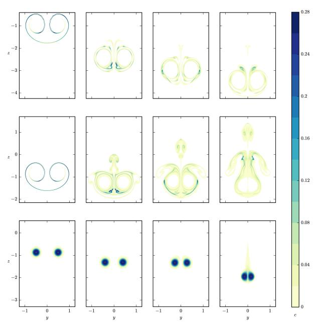
Figure 6: Evolution of the passive scalar field over time. From top to bottom:  $\text{Fr}^{-1} = 0.2$ ,  $\bar{b}_{\text{jet}} = 0.16$ ;  $\text{Fr}^{-1} = 1$ ,  $\bar{b}_{\text{jet}} = 0.16$ ;  $\text{Fr}^{-1} = 1$ ,  $\bar{b}_{\text{jet}} = 0.79$ . From left to right:  $t = \tau_0$ ,  $2.5 \tau_0$ ,  $3 \tau_0$ ,  $3.5 \tau_0$ .
