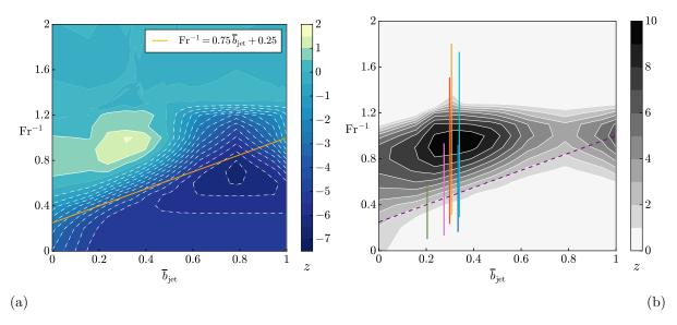
Figure 8: (a) Mean altitude of the plume and (b) difference between the mean altitude of the plume and that of the vortices at  $t = 5 \tau_0$  as a function of  $Fr^{-1}$  and  $\bar{b}_{jet}$ . The purple dashed line on the right panel corresponds to the orange line on the left panel.
