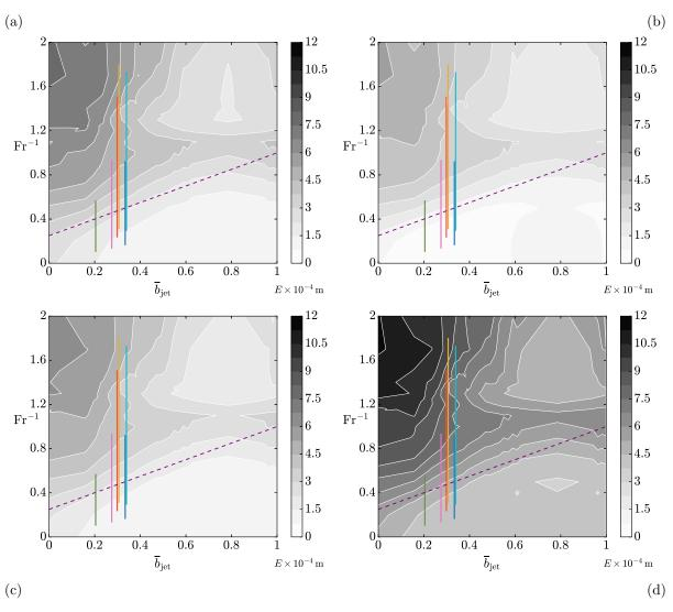
Figure 10: Total extinction E for (a) RH = 140% and (b) RH = 120% at  $t = 5\tau_0$ . In (c) only half of the soot are nuclei and (d) considers the emission index of water for a liquid hydrogen engine for RH = 140%. The vertical lines represent the range of possible parameters for a selection of twin-engined aircraft (from left to right): CRJ, B737, B777, A330, A320, B787. For the purple dashed line legend, see figure 8
