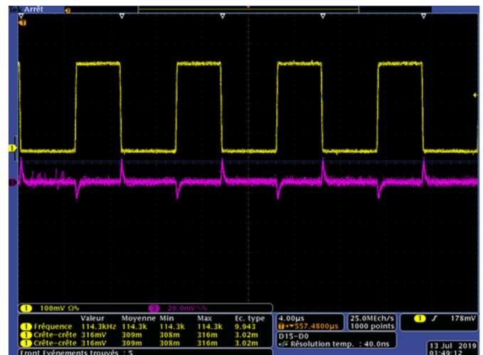
Fig. 25. Experimental result with  $80\text{fC}$  input charge applied which correspond to  $U_1=200\text{mV}$ . AFE response voltage is  $U_2=20\text{mV}$ .
