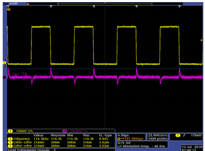
Fig. 25. Experimental result with 80fC input charge applied which correspond to U_1=200mV . AFE response voltage is U_2=20mV .
