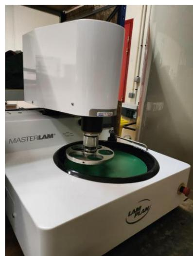
Figure 5: Picture of the polishing device MASTERLAM 1.0 from LAM PLAN.
