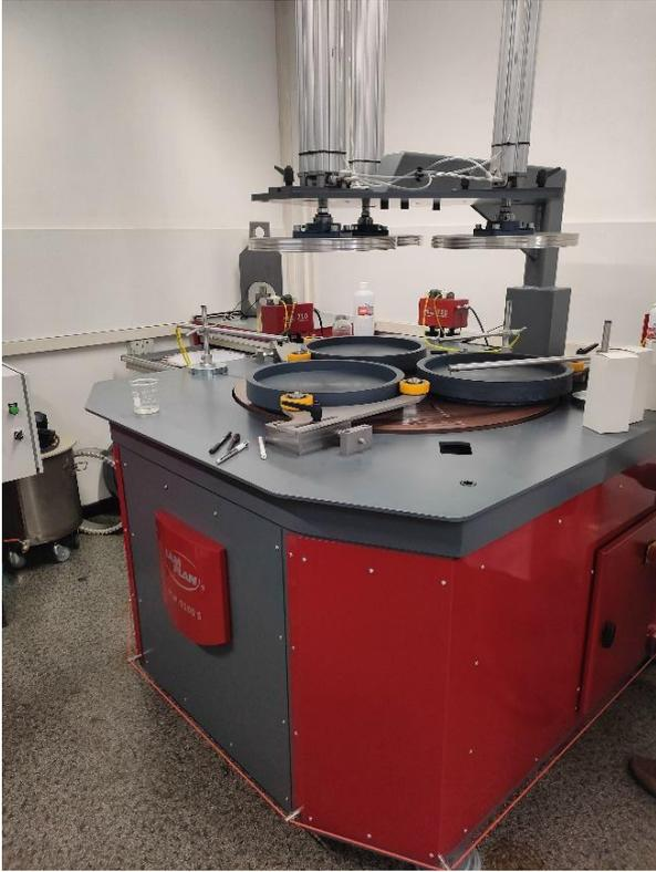
Figure 20: Photograph of the polishing machine MM.9100S in operation at LAM PLAN company.
