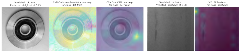
Figure 2: Example interpretability maps computed on misclassified images, first from the casting defect dataset (left side: raw picture, then heatmaps for CNN Occlusion and CNN GradCAM), and from the NEU-DET dataset (right side: raw picture, then heatmap from ViT LRP).
