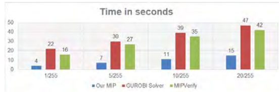
Figure 3: Computational Time for robustness problems averaged over 100 instances according to the intensity of the attack (maximum disturbance allowed in infinite norm)
