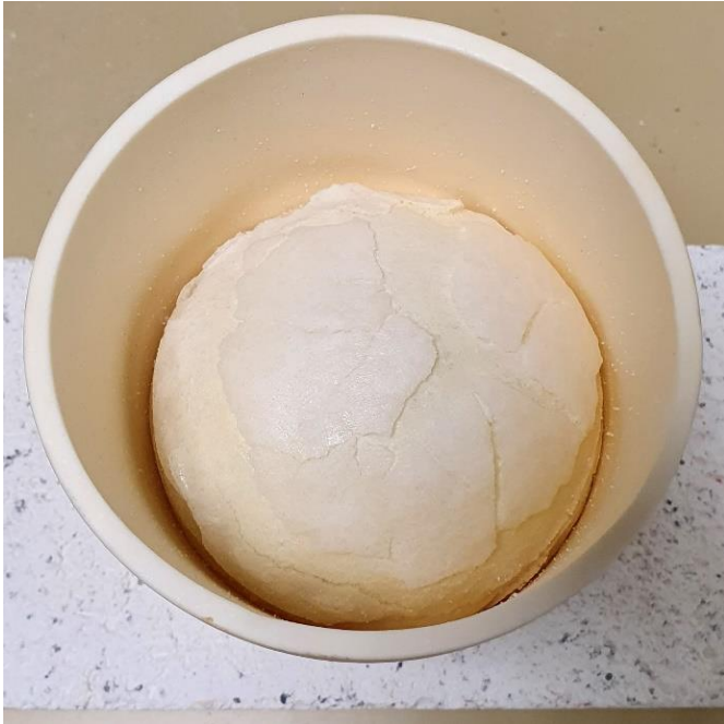
FIG 1. MgO-Y 2 O 3 nanocomposite powder (10g) obtained after the 600-1200°C heat treatment (thermal sol-gel process). Inner diameter of the crucible = 90mm. (1-column fitting image)
