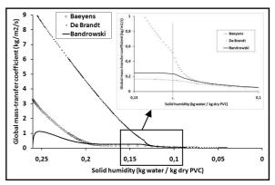
Fig. 8: Evolution of the global mass-transfer coefficient with the solid humidity
