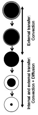
Fig. 1: Particle drying
