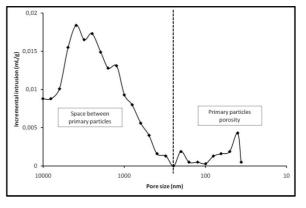
Fig. 3: pores size distribution of PVC's particle
