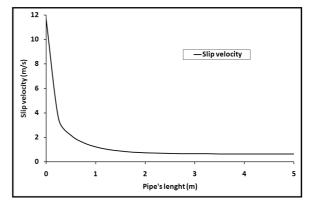
Fig 7: Evolution of slip velocity along the dryer
