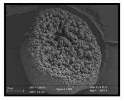
Fig 2: SEM picture of a PVC particle
