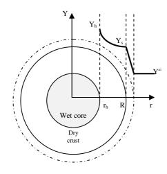
Fig. 4: The shrinking core model
