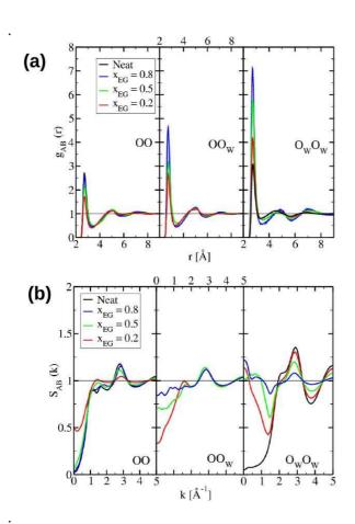
Fig.3 Oxygen-oxygen correlation functions (a) and structure factors (b) for the aqueous-ethanediol mixtures. The diol concentrations are shown in blue for x = 0.2, green for x = 0.5 and red for x = 0.8. Pure solvent data is shown in black. Left panel for the oxygen atoms of the diol, middle panel for the cross correlations and right panel for the oxygens atom of water.
