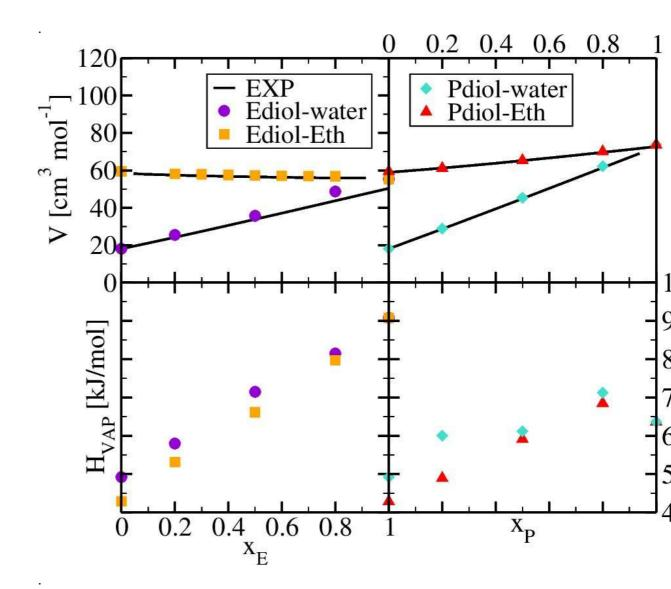
Fig.10 Thermodynamic properties. Volumes in (a) and (b), enthalpies in (c) and (d). Black line for experimental data [62, 63, 64, 65], purple circles for aqueous-ethanediol, gold squares for ethanol-ethanediol, cyan symbols for aqueous-propanediol and red triangles for ethanol-propanediol.
