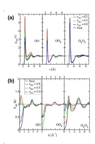
Fig.5 Oxygen-oxygen correlation functions (a) and structure factors (b) for the ethanol-ethanediol mixtures, with same colouring conventions as in Fig.3.
