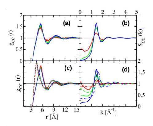
Fig.7 Central methylene group correlations( (a) and (c) and structure factors( (b) and (d) ) for the aqueous-propanediol (upper row (a) and (b)) and ethanol-propanediol (lower row (c) and (d)). The line colors correspond to different concentrations, with the same convention as Fig.3. Full lines for the methylene of ethanediol and dashed for that of ethanol.
