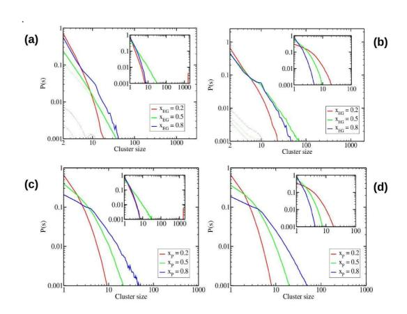
Fig.2 Clusters distributions of the diol oxygen sites (main panels) and solvent oxygen sites (insets), versus the cluster size, for (a) the waterethanediol mixtures, (b) the ethanol-ethanediol mixtures, (c) the waterpropanediol mixtures and (d) the ethanol-propanediol mixtures. The diol concentrations are shown in red for x = 0.2, green for x = 0.5 and blue for x = 0.8. The thin dotted line in (a) and (b) are explained in the text.
