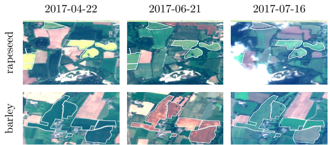
(b) Images of BARLEY and RAPESEED fields on three selected dates. The model stopped the classification of RAPESEED fields end of April when the characteristic yellow blossoms were visible, shown in the April 22nd image. BARLEY field classifications were stopped end of June during the harvest, as visible in June 21st, where bare soil is visible on the field parcels.
