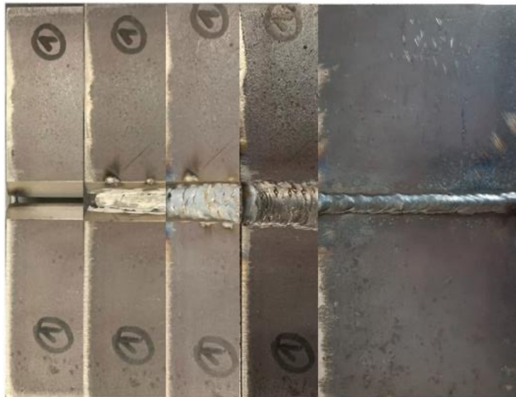
Figure. 2: different steps of welding
