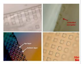
**Figure 4.** Example of PDMS-based hierarchical microstructured material used for tactile sensing. Adapted with permission from Desmulliez (2018).
