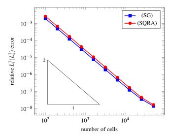
Fig. 4: Convergence of the schemes under space grid refinement, ( $\lambda^2=10^{-2}$ ).
