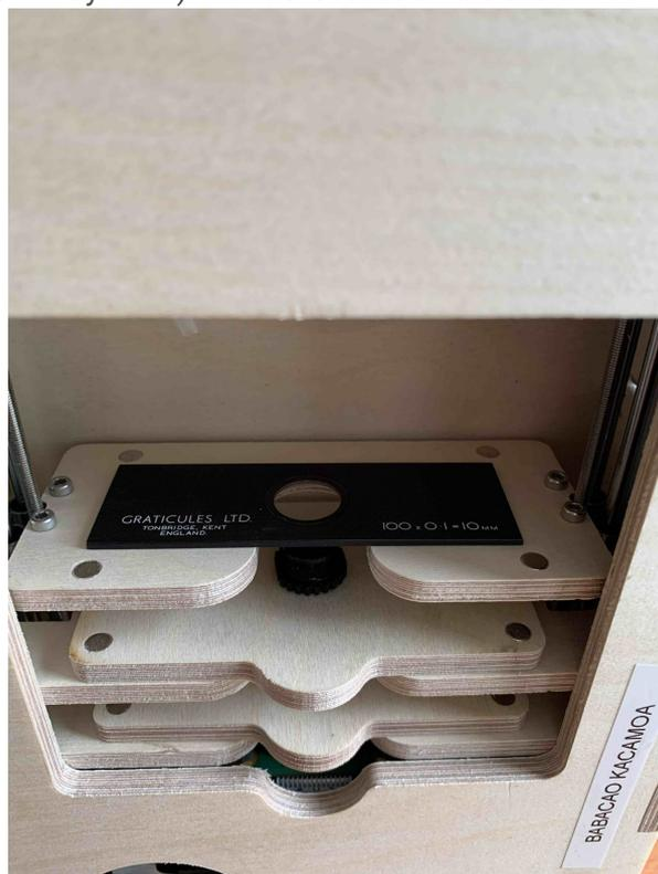
placing the calibration slide (once removing the flowcell)
