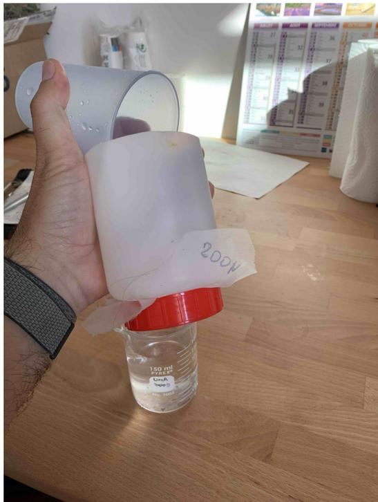
filtration through a 200µm mesh
