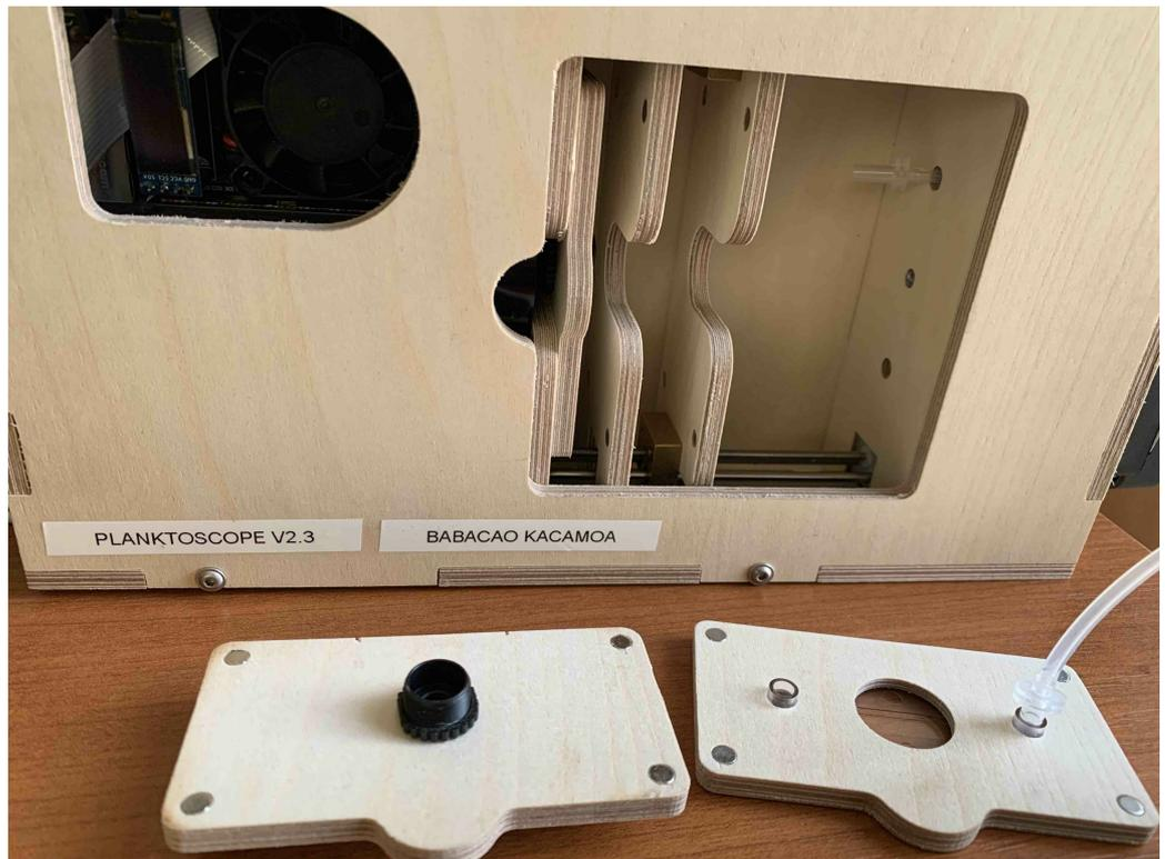
objective lens and flowcell removed
