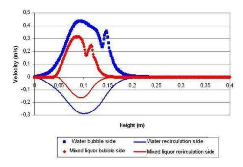
Axial velocities on vertical lines located in the middle of the initialisation of the bubble and at the opposite side of the membrane obtained by CFD
