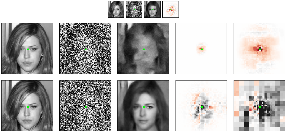
Figure 4: Denoising examples. Each row shows clean image, noisy image, denoised image, and the adaptive filter (one row of the Jacobian of the end-to-end denoising transformation) used by the denoiser to estimate a specific pixel, indicated in green. The heat-map ranges from red for most negative to black for most positive values. In the last two rows, the last column shows an enlargement of this adaptive filter, for enhanced visibility. Images are displayed proportional to their sizes. Top row: 40 \times 40 images estimated with a CNN denoiser with RF 40 \times 40 . Second row: 160 \times 160 images estimated with a CNN denoiser with RF 43 \times 43 . Third row: 160 \times 160 images, estimated with the proposed conditional multi-scale denoiser of Figure 2. The denoiser uses a 40 \times 40 RF for the coarsest scale, and 13 \times 13 RFs for conditional denoising of subsequent finer scales.
