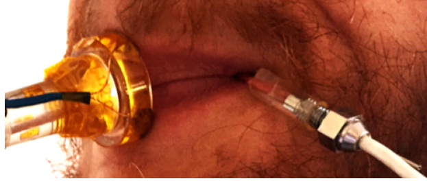
Figure 1. (Color online) Measurement of the mouth pressure through a thin tube inserted at the corner of the mouth.
