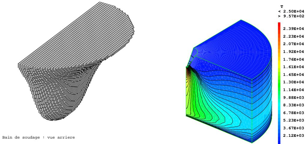
Figure 2: Discretization grid for `Weld_pool(cst)` problem (left) and temperature distribution for `Arc_3D_b` problem (right); in this latter case, the viscosity is related to the temperature via the relation pictured in figure 3.
