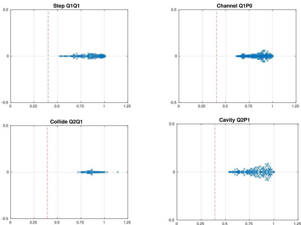
Figure 4: Representation of the spectrum of  $A_{\text{sp},c}^{-1}A_c$  in the complex plane for different finite element discretizations and different problems: the blue “ $\times$ ” represent the eigenvalues, while the vertical dashed red lines cross the real axis at the value  $x = 1/(1 + \gamma_{\mathbf{u}})$  of the lower bound (5.4).
