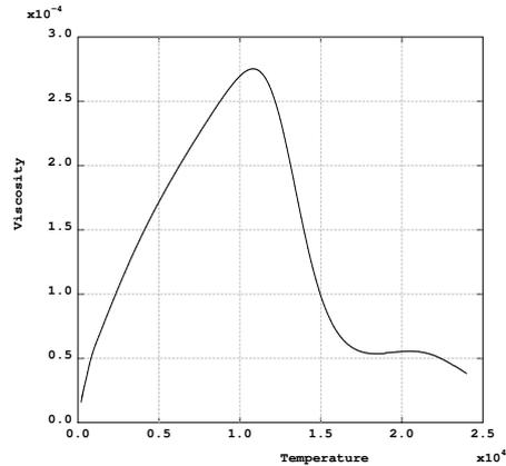
Figure 3: Viscosity of argon as a function of temperature used in `Arc_2D`, `Arc_3D_a`, and `Arc_3D_b` problems.
