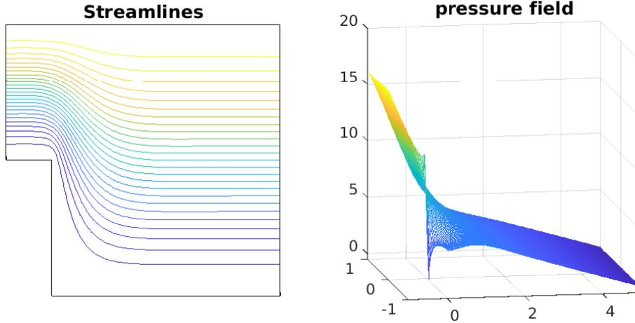
Figure 1: Streamlines and pressure field for the `Step` problem.
