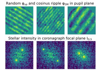
**Figure 11. Top:** Phase resulting from the sum of a random aberrations  $\phi_{\rm up}$  and one cosine  $\phi_{\rm DM}$  applied on the DM for three frequencies and directions. **Bottom:** Associated coronagraphic images  $I_{D,S}$ .
