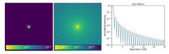
**Figure 2. Left and center**: Normalized point spread function for a full pupil telescope of diameter D with two different color-bars. **Right**: Intensity as a function of angular separation normalized to its maximum.
