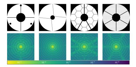
**Figure 5.** Left to Right: Apertures (top) and associated normalized intensity of the PSF (bottom) for the HST, VLT, JWST and ELT (in plane B). For the ELT and JWST the inner and outer edge of the pupil were made circular which is customary when designing coronagraphs. Apertures were re-created using [59].
