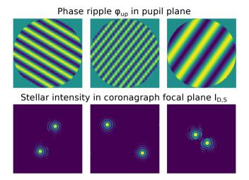
**Figure 8. Top:** Sine phase  $\phi_{up}$  for three spatial frequencies and directions in the pupil plane. **Bottom:** Associated coronagraphic image  $I_{D,S}$ .
