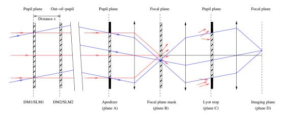
**Figure 10.** Stellar coronagraph associated to two active optical corrector (deformable mirror, DM, or spatial light modulator, SLM). See Figure 3 and text for details.
