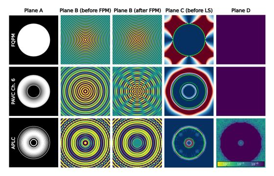
**Figure 6.** Same as Figure 4 for three other coronagraphs. **From top to bottom:** Numerical simulations of the light distribution in plane A to plane D for a Classical Lyot coronagraph; a four-quadrant phase mask [42, FQPM]; a Polynomial apodized Vortex coronagraph [73] of charge 6 designed for a central obscuration of 36% of the pupil; an APLC [70] designed for a central obscuration of 17% of the pupil.
