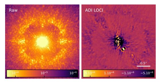
Figure 16. Left: Raw coronagraphic image recorded by SPHERE/IRDIS with 2s exposure and dominated by a smooth halo at the center and stellar speckles elsewhere. Right: Processed image by LOCI of 200 raw coronagraphic images recorded with angular differential imaging. The exoplanet  $\beta$ -Pictoris b is located on the bottom-right of the star. Color bars are in normalized intensity.
