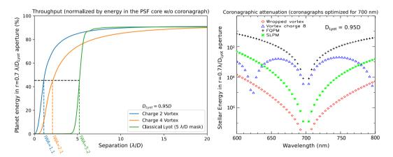
**Figure 9. Left**: Numerically simulated throughput for classical Lyot, vortex charge 2 and 4 coronagraphs [43]. Vertical dashed lines give the IWA for each coronagraph. **Right** (adapted from [46]): Numerical simulations of monochromatic performance as a function of wavelength for wrapped vortex [46], charge 8 vortex [43], four-quadrant phase mask [42] and six level phase mask [60] coronagraphs optimized at 700 nm.
