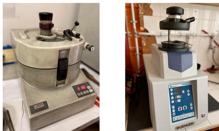
Figure 3. Milling (left) and hot compaction (right) of the mixture.
