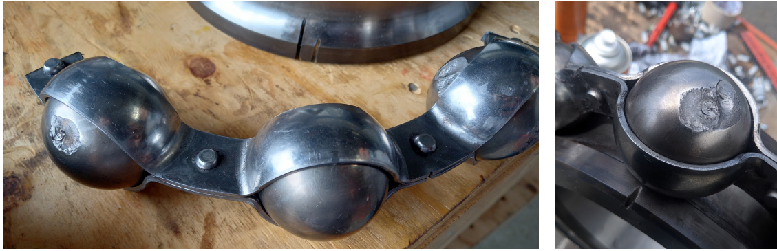
Figure 7: Rolling elements of the damaged bearing.
