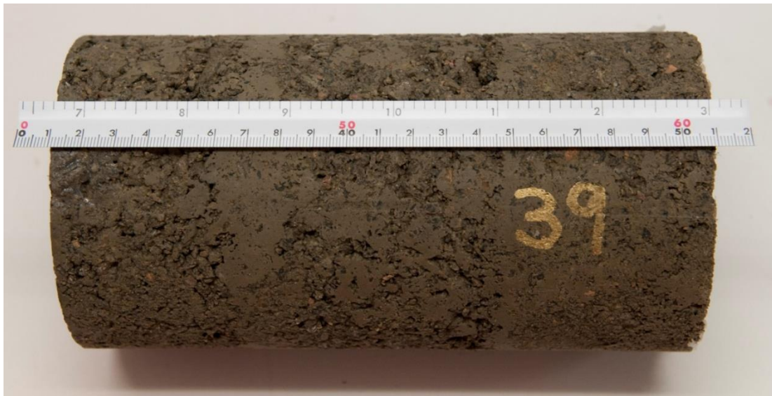
Figure 3. Sample body 39. The sample body contains a mixture of all five binders. In the photo, three different subsets can be discerned.
