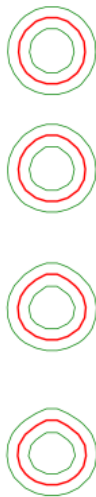
Figure 1: Successive representations of the interface of the sedimented Eulerian droplet falling within a box. Interface is shown at distances \phi(x) = [-\Delta x; 0; \Delta x] , in green, red, green, respectively. Results are obtained at D_D/\Delta x = 6.4 at t/\tau_p = [0, 1.8, 3.6, 4.5] , from top to bottom.
