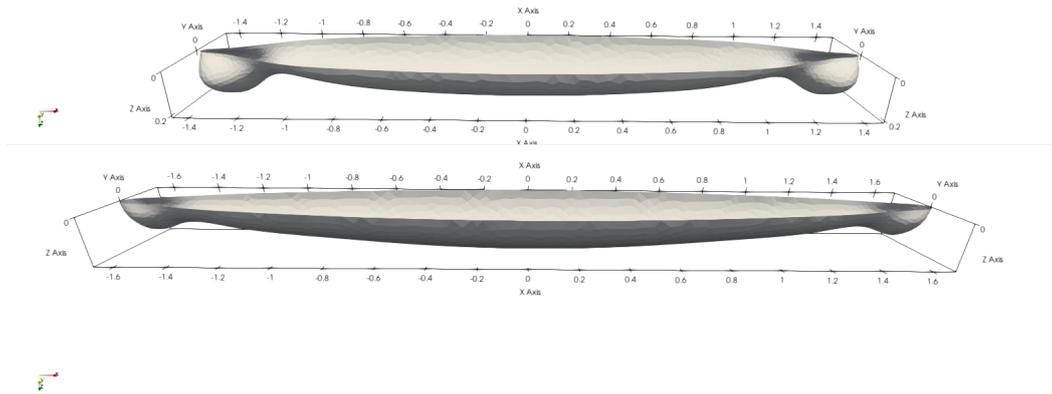
FIGURE 19. The optimal hulls for minimizing the total water resistance at  $Fr = 0.73$  ( $\bar{u}$ , top) and for minimizing the expectation of the total resistance for  $Fr \in [0.6, 1]$  with  $\nu$  uniform ( $u^*$ , bottom).
