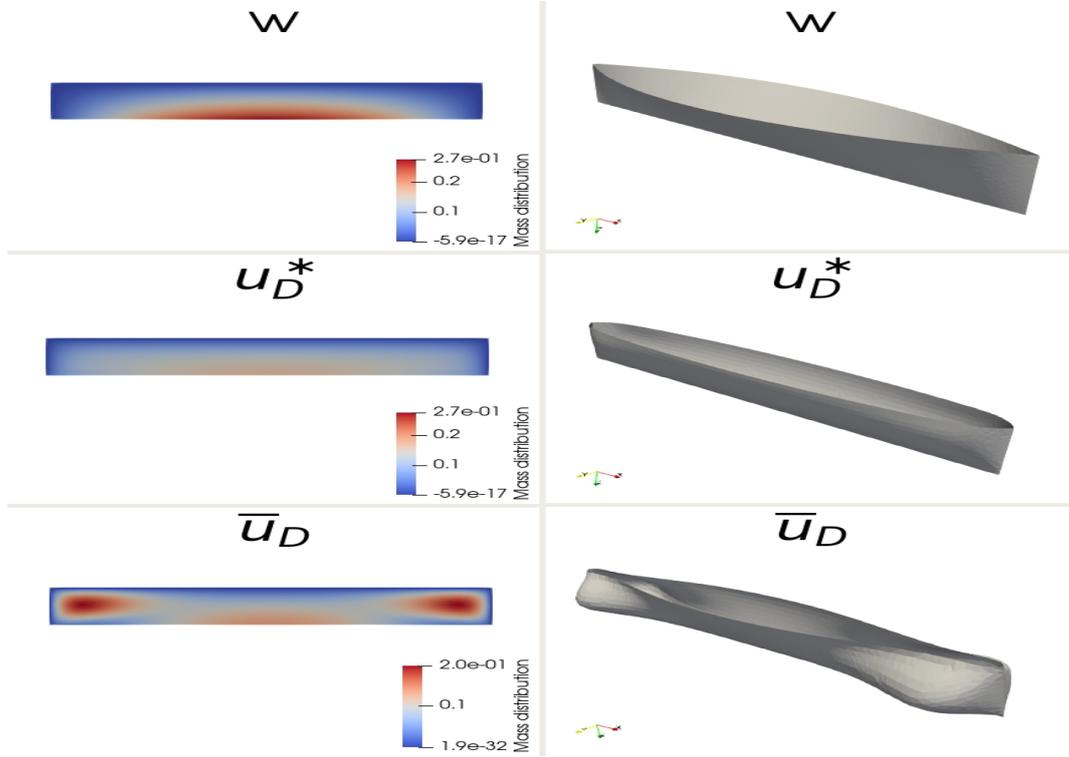
FIGURE 5. Mass distribution (left), and 3D results (right) of the Wigley hull  $w$  (top), the optimal hull  $u_D^*$  (middle, optimized for a uniform distribution of  $V$ ) and the optimal hull  $\bar{u}_D$  (bottom, optimized for  $\alpha = \mathbb{E}[\nu]$  with  $V$  uniform).
