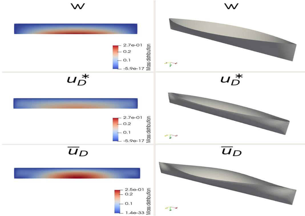
FIGURE 3. Mass distribution (left), and 3D results (right) of the Wigley hull  $w$  (top), the optimal hull  $u_D^*$  (middle, optimized for a uniform distribution of  $\nu$ ) and the optimal hull  $\bar{u}_D$  (bottom, optimized for  $\alpha = \mathbb{E}[\nu]$  with  $\nu$  uniform).
