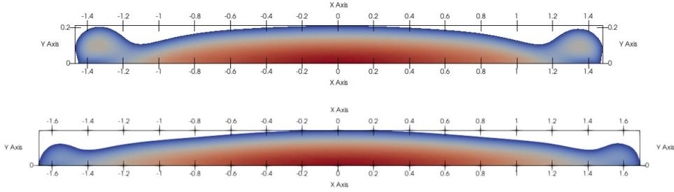
FIGURE 18. The optimal domains for minimizing the total resistance at  $Fr = 0.73$  (top) and for minimizing the expectation of the total resistance for  $Fr \in [0.6, 1]$  with  $\nu$  uniform (bottom).
