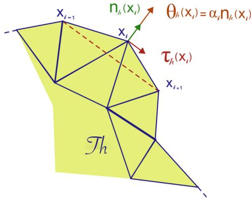
FIGURE 7. Discrete setting around a vertex  $\mathbf{x}_i$
