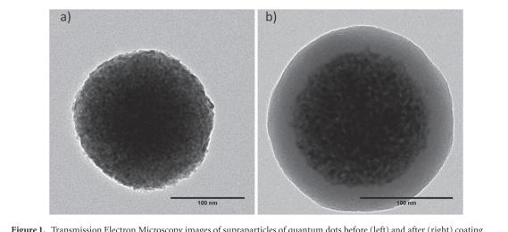
**Figure 1.** Transmission Electron Microscopy images of supraparticles of quantum dots before (left) and after (right) coating with silica.
