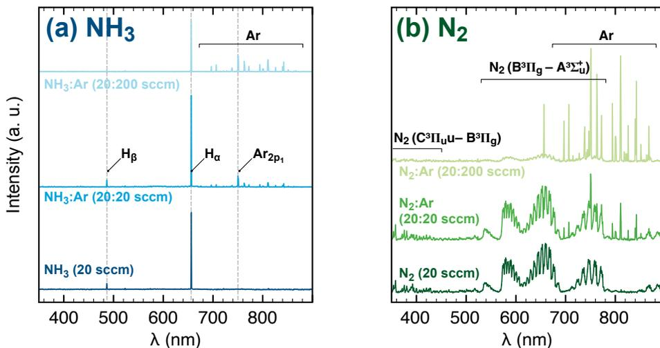
FIG. 4. OES spectra of (a)  $pl\text{-NH}_3$  and (b)  $pl\text{-N}_2$  pure or mixed within different Ar flows. Measurements are taken at the plasma generator window with  $P_{\text{plasma}} = 300 \text{ W}$  using an acquisition time of 44 ms. The peaks have been identified according to literature<sup>48–50</sup>.
