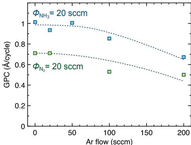
FIG. 5. Influence of dilution in Ar on both  $pl\text{-NH}_3$  and  $pl\text{-N}_2$ .  $\phi_{\text{NH}_3}$  and  $\phi_{\text{N}_2}$  are constant at 20 sccm.
