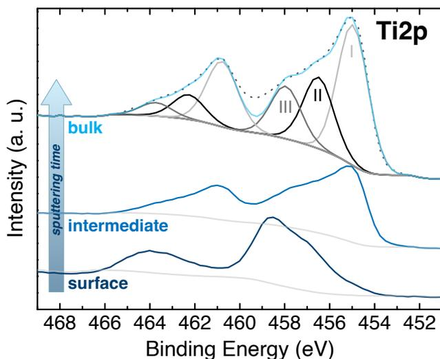
FIG. 11. XPS spectra of Ti2p peak from *pl*-NH<sub>3</sub> TiN film at different sputtering durations.
