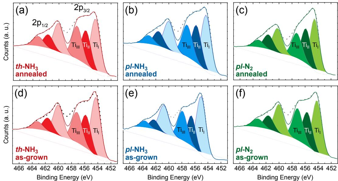
FIG. 10. Ti 2p XPS peaks from (a) *th*-NH<sub>3</sub>, (b) *pl*-NH<sub>3</sub> and (c) *pl*-N<sub>2</sub> processes before and after annealing at  $T_{\text{an}} = 700^\circ\text{C}$  (d,e,f), respectively.
