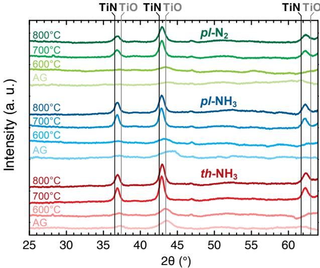
FIG. 12. XRD patterns of as-grown layers and their evolution with annealing temperature for the three deposition routes. Annealing in N<sub>2</sub>, NH<sub>3</sub> and H<sub>2</sub> mixture for 5 min at  $T_{\text{a}} = 600, 700$  and  $800^\circ\text{C}$ . Black and gray vertical lines correspond to TiN and TiO references, respectively.
