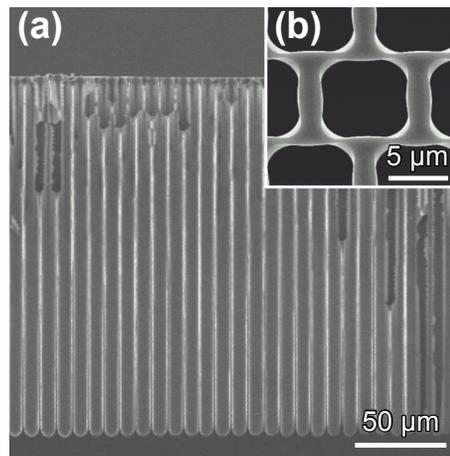
FIG. 1. SEM observations of bare ordered macropores: (a) cross section and (b) top view. Pores opening and length are respectively around 7 and 215  $\mu\text{m}$ , that corresponds to an aspect ratio of 1:30.
