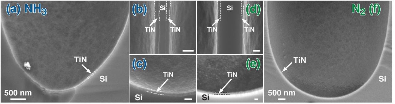
FIG. 9. SEM cross sections of porous Si coated by TiN films: (a,b,c)  $pl$ -NH<sub>3</sub> and (d,e,f)  $pl$ -N<sub>2</sub>. (a,f) show general views of pore tips while (b,e) and (c,d) show high magnification images of a single wall at half depth of the pore and at the pore tips, respectively. Scale bars in (b,c,d,e) correspond to 100 nm. Expected 50 nm-thick TiN layers grown at  $T_{ALD} = 200^\circ\text{C}$ .
