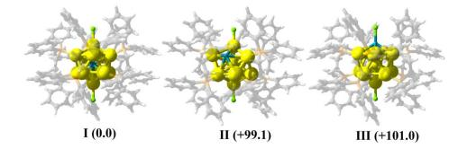
**Figure 1.** Relaxed structures of the three isomers **I-III** of  $[OsAu_{12}Cl_2(dppe)_5]$  (2). Relative energies are given in brackets (kcal.mol<sup>-1</sup>). Os atom is in blue.
