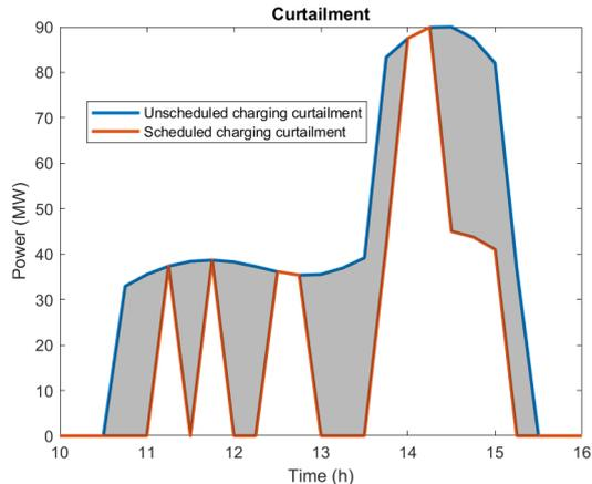
Fig. 2. Curtailment cut. Uncoordinated vs coordinated charging scenario
