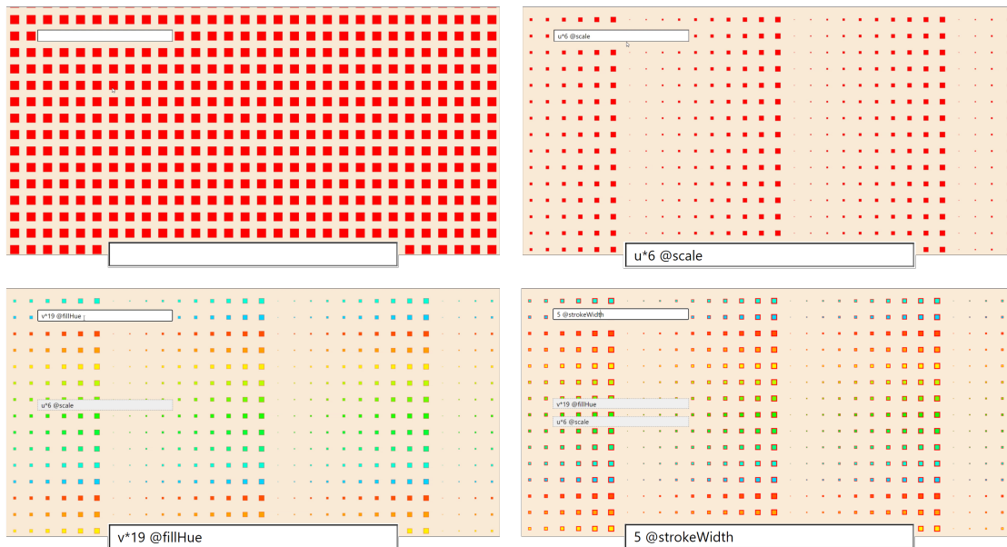
Fig. 3. VectorPattern interface. The drawn pattern is computed based on formulae written in a text field. The application starts with an empty field and a default pattern (red squares). We show here successive formulae written by the user. First a formula function of u (horizontal coordinate) is applied to the scale, using the @scale keyword. Then a formula function of v (vertical coordinate) is applied to the fillHue property. And finally a simple constant is applied to the strokeWidth.
