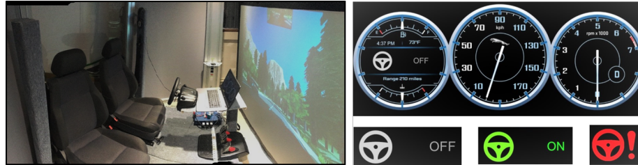
Fig. 2. Left : The driving simulator. Right : View of the dashboard and the icons indicating the driving mode.
