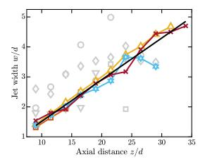
FIG. 10. Peak width w as a function of the axial distance z (both quantities are normalized by the nozzle diameter d). Color symbols: points with  $L_0 > L_t$ , i.e. data sets A2 (in part), A3, B3, and B4, collectively named high set; gray symbols: remaining points, with  $L_0 \le L_t$ , i.e. data sets A1, A2 (in part), B1 and B2, collectively named low set. Note that the symbols are as in Fig. 9, regardless of their color; black line: linear fit, Eq. (10).
