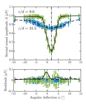
FIG. 4. Top panel: two sets of 30 sweeps (points) across the jet axis, obtained at 1.65 K and 776 mW (data set A3) for z/d=9.0 and 31.5, as indicated in the figure. Solid and dashed black lines: ensemble-averaged data used for the calculation of the quantized vortices' density. Dot-dashed black line: deflection offset  $\alpha_0 \approx 1.9^\circ$ , Eq. (7). Bottom panel: residuals (points) and standard deviations (lines) corresponding to the data displayed in the top panel.
