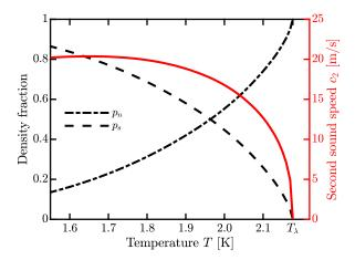
FIG. 1. Left axis: temperature dependence of the density fractions of the normal  $(p_n, \text{dot-dashed line})$  and superfluid  $(p_s, \text{dashed line})$  components of He II. Right axis: temperature dependence of the second sound speed (solid line).  $T_{\lambda} \approx 2.2 \text{ K}$  denotes the superfluid transition at the saturated vapor pressure. Data from Ref. DB98.
