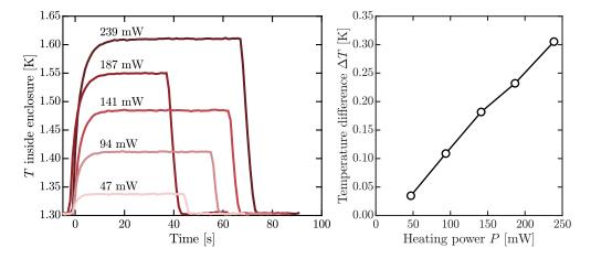
FIG. 6. Left panel: temperature inside the heater enclosure as a function of time. The bath temperature is kept constant at 1.30 K and the heater is supplied by a constant heating power (specified near each curve) from approximately zero time. Right panel: steady temperature difference  $\Delta T$  between the enclosure and the <sup>4</sup>He bath as a function of the heating power P.
