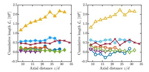
FIG. 11. Cumulative length  $\mathcal{L}_z$  of quantized vortices per unit height as a function of the normalized axial distance z/d. Left panel: right-hand side of Eq. (15), computed using the experimentally obtained values of  $L_0$  and w. Right panel: result of the numerical integration of the right-hand side of Eq. (11) as discussed in the text. Colors as in Fig. 9.
