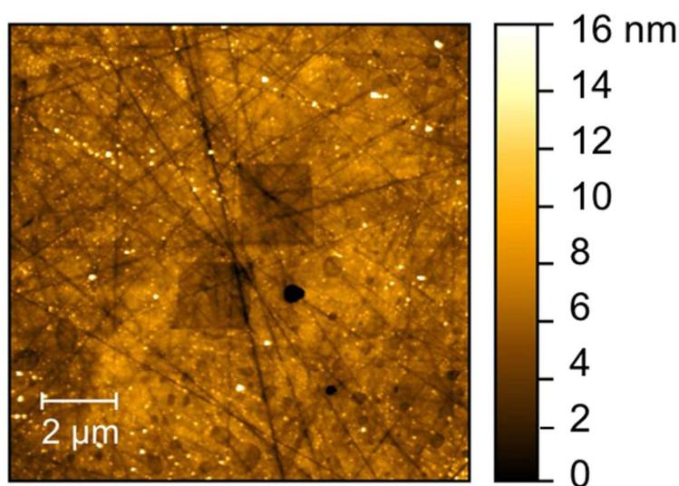
Figure 9: 10x10 mm<sup>2</sup> topography Image after 2 nanoshaving experiments performed in situ (100°C, PAO 4 + 1 % wt PFM) outside track.
