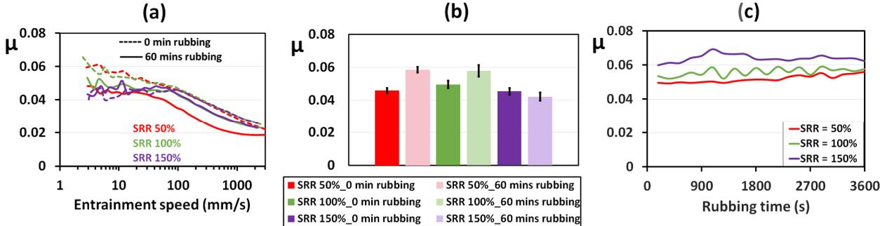
Figure 4: In (a) the Stribeck curves of the MTM tests at 100 °C as a function of SRR for the lubricant (PAO 4 + 1% wt PFM). In (b) the histograms of the friction coefficients averaged over low speeds between 3 and 10 mm/s. The rubbing curves between Stribeck curves in (c).
