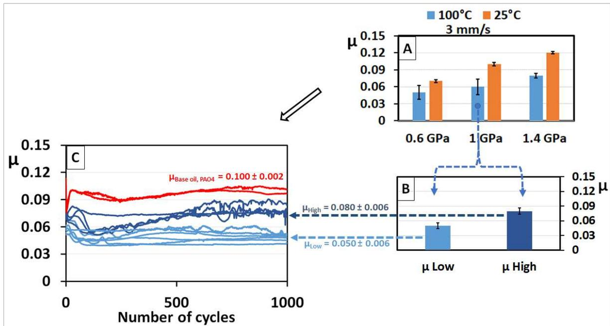
Figure 6: In A the histograms of the friction results on the reciprocating tribometer at 3 mm/s as described in figure 5. In B, the test conditions (3mm / s, 1GPa and 100 ° C) are transformed as a function of friction level into 2 different histograms. In C, friction curves of PAO 4 in red and corresponding friction curves.
