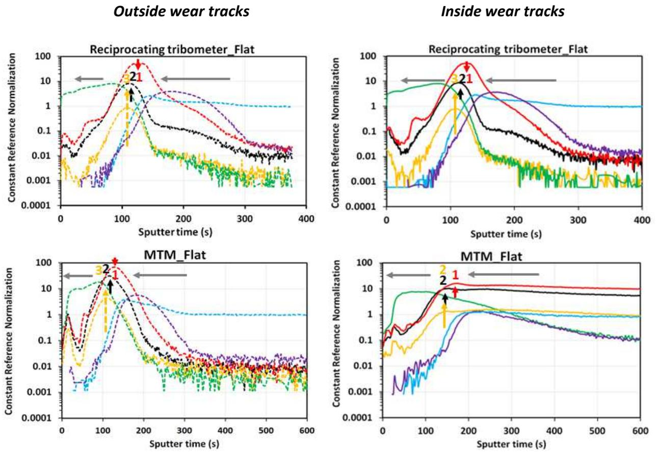
Figure 8: On left, Tof-SIMS profiles obtained outside the flat friction tracks (dotted line) and on right, Tof-SIMS profiles obtained inside the flat friction tracks in solid lines for MTM and reciprocating friction test specimens.
