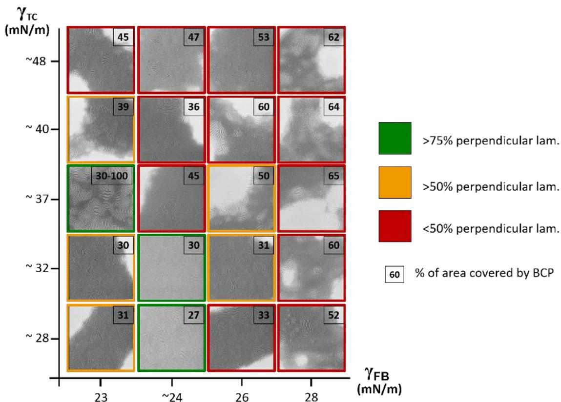
Figure 7. Cartography for the self-assembly of L-DBS18 coated on the FB materials as under-layers, as function of the surface energy of the various TCs. Cross-linking of the TCs by UV ( $180 \text{ mJ.cm}^{-2}$ ) followed by a  $90^\circ\text{C}$ -3 minutes bake. Thermal bake performed at  $170^\circ\text{C}$ -5mins to limit the dewetting of the BCP. Magnification  $\times 100000$  with field area of  $1.35 \mu\text{m} \times 1.35 \mu\text{m}$ .
