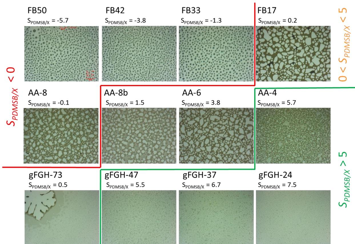
Figure 2. Optical microscope images of the surface of our BCP film after thermal annealing at 170°C for 3 minutes with no top-coat. The calculated spreading factor  $S_{PDMSB/X}$  of homo-PDMSB on the surface (in  $mN.m^{-1}$ ) is reported for each surface (assuming a symmetric parallel wetting). Magnification  $\times 100$  with field area of  $125 \mu m \times 94 \mu m$ .
