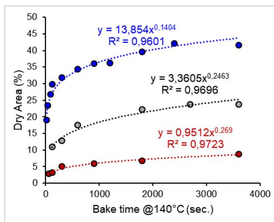
Figure 5. Dewetting kinetics of a symmetric BCP layer with a partially UV crosslinked FGH37 TC and a AA-8 neutral UL (UV dose: blue: 45 mJ.cm<sup>-2</sup>, grey: 90 mJ.cm<sup>-2</sup>, red: 180 mJ.cm<sup>-2</sup>). The area of dry holes in the BCP layer is monitored as function of self-assembly bake time. The dotted lines are the ones for the power-law best-fit of each data set. 7 randomly taken SEM images are used for each sample (one sample per time increment).
