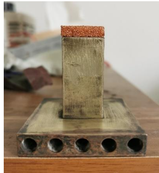
Fig. 4. Metal foam soldered to a heated copper block.
