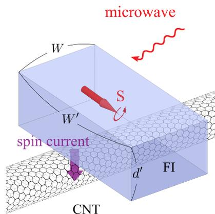
FIG. 1. Magnetic junction composed of a ferromagnetic insulator (FI) and a single-wall carbon nanotube (CNT). The dimension of the FI is  $W \times W' \times d'$ .
