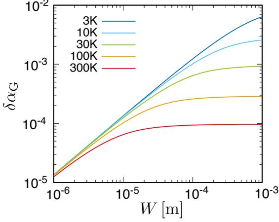
FIG. 3. Junction-length dependence of increase in the Gilbert damping,  $\delta\alpha_{G,1}$ , for a clean interface ( $J_1 \gg J_2$ ).
