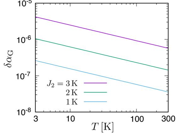
FIG. 4. Temperature dependence of increase in the Gilbert damping,  $\delta\alpha_{G,2}$ , for a dirty interface ( $J_2 \gg J_1$ ). The three lines correspond to  $J_2 = 1, 2$ , and 3 K, respectively.
