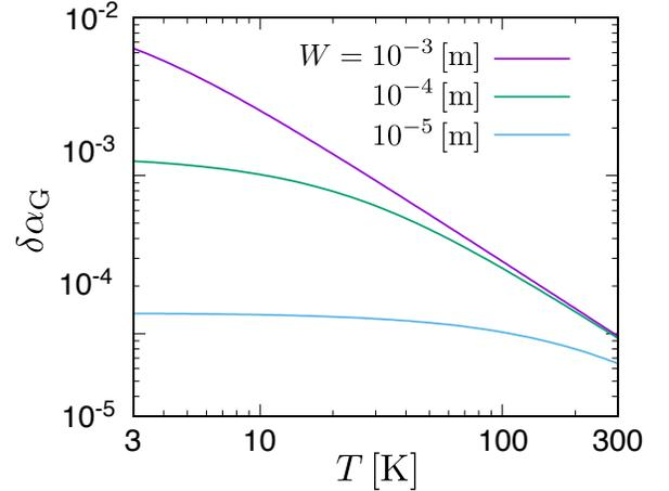
FIG. 2. Temperature dependence of increase in the Gilbert damping,  $\delta\alpha_{G,1}$ , for a clean interface ( $J_1 \gg J_2$ ).
